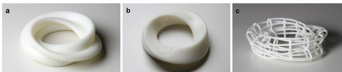
Figure S1 | 3D prints of the torus-knot topology. Models of the torus-knot beam topology of Fig. 1, printed in 3D using resin-based stereolithography (SLA) on a Formlabs Form 2 printer. 3D Prints: Xavier Menino (ICFO); Image Credits: © ICFO.
